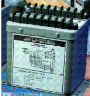
When the kW sensor closed loop control option is implemented with the GECO·Lean Burn control, the generator output power signal is required at terminals 55 and 60. This is a 4–20 mA signal scaled appropriately for the generator size. There are many watt transducers that can be used.
