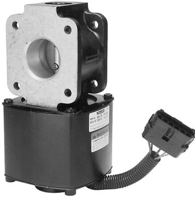
[P/N 8235-142, 8235-160 or 8235-154] The Flo-Tech™ electrically-actuated valve controls fuel pressure to the air/fuel mixer. It is a butterfly-type valve available in 33, 48, 60, 68, and 75 mm bore sizes for various applications. The valve position responds proportionally to the position command signal.
