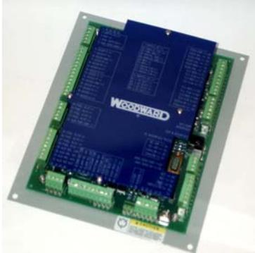
**[P/N 9907-866]** The circuit board includes the microprocessor controller and all associated electronics for power regulation, signal inputs and filtering, controlled outputs, and communications. All system connections are made directly to the board through plug-in terminal strips and connectors. The board also includes a status indicator light, control mode switch, and a fuse.
