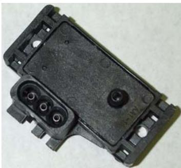
The Manifold Absolute Pressure sensor (MAP) is used by the controller to measure the intake manifold pressure. It is an absolute pressure sensor with a 300 kPa (43.5 psi) range and a 0–5 Vdc output signal. Like the UEGO sensor, it was developed for the automotive industry.
