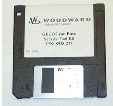
The PC service tool software is executed on a Microsoft DOS compatible PC. When the COM1 or COM2 ports of the PC are connected to the RS-232C port of the GECO™·Lean Burn control (DB9 connector), the service tool software will provide monitoring and display of the set-up and tuning parameters of the GECO·Lean Burn control application software.
