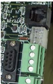
The 6-pin Molex connector next to the RJ12 connector provides a connection to a panel or remotely mounted LED display of power, alarm, and shutdown status. See the section below in this chapter titled "LED Status Indicators".
