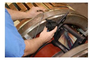
regions of the machine. But even without a borescope, an experienced inspector can determine quite a lot simply by the looking at the interior of the generator.
