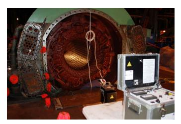
More extensive electrical tests are also now possible. Specifically, d.c. leakage tests and high potential tests can be performed on each phase of the stator. These tests can help determine the long term condition of the ground wall system by trying to indentify incipient faults during an inspection outage, and before a catastrophic failure occurs when the machine is in service. This approach
