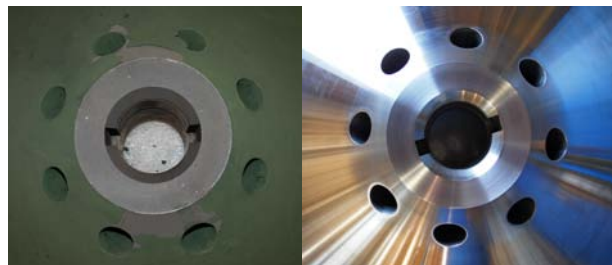
(Left) A CRV Valve Disk with its bore and face nitrided. Note the off-green masking on the remainder of the disk. (Right) The same valve disk after polishing and before magnetic particle inspection.
